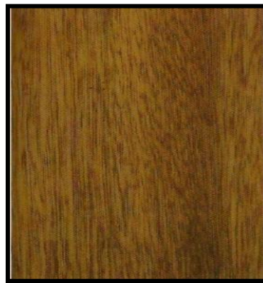
Figure 1.2. Wood characteristic of Lauraceae. Adapted from “Common Commercial Timbers of Peninsular Malaysia,” by K. S. Gan and S. C. Lim, 2004, Research Pamphlet No. 125 , p. 38.
