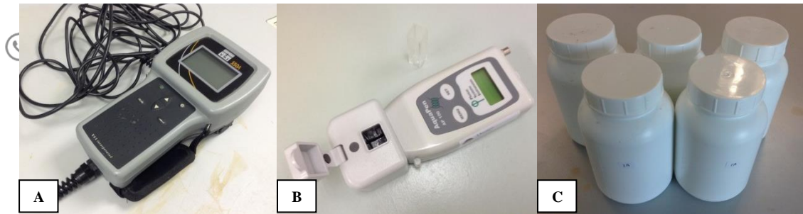
Figure 3.3. Water sampling equipments. (A) YSI 550A portable probe, (B) AquaPen-C AP-100 and (C) HDPE bottles
