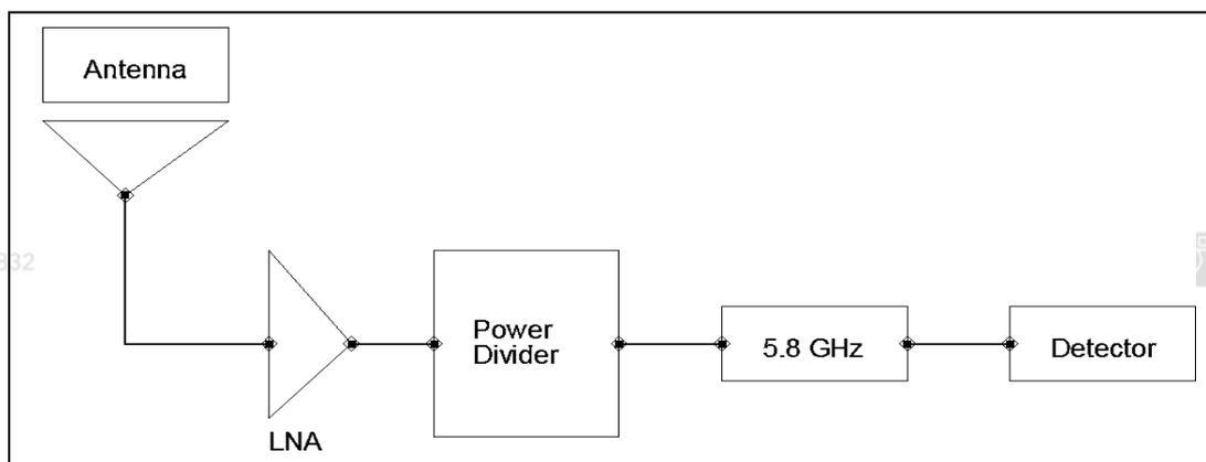
Figure 1.1. Front-end receiver block diagram
